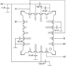
Fig. 5 Recommended schematic. The supply filter capacitor should be 1μF or more. The capacitors 100nF and 10nF should be placed close to the device. Connections A1, B1, A2, B2, I2 are required for programming and linearization.
